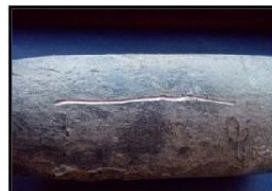
Lead pipes are dull gray and very soft and look like a new nickel when scratched
